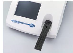
Pic. 18: Check alignment of notches
