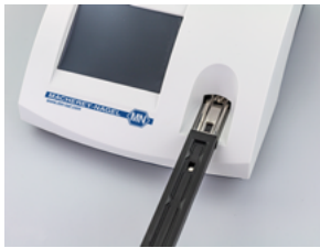
Pic. 17: Reinsertion of the test strip holder
